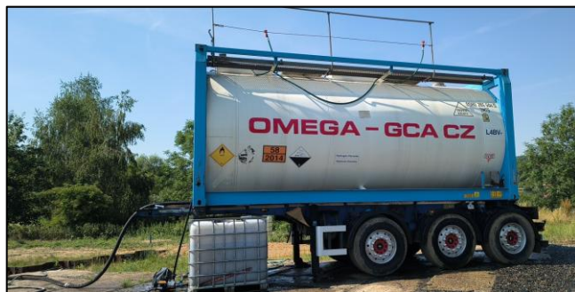
Obr. 4 a 5 Bioreaktor pro aplikaci biodegradace in situ a isokontejner na \text{H}_2\text{O}_2 pro chemickou oxidaci ISCO Fig. 4 and 5 Bioreactor for in situ biodegradation application and \text{H}_2\text{O}_2 isocontainer for chemical oxidation ISCO
